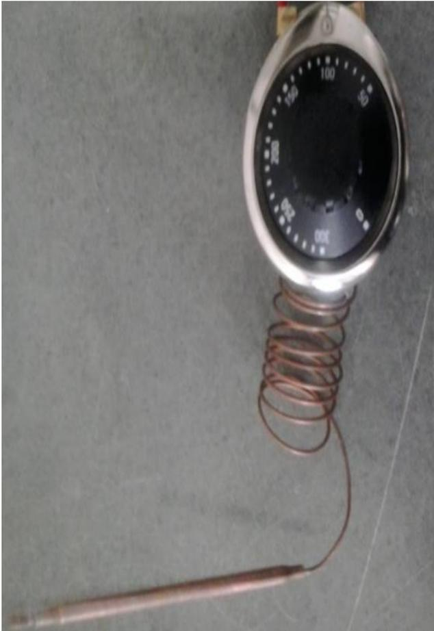
**Fig.12 Temperature sensor (thermostat)**
