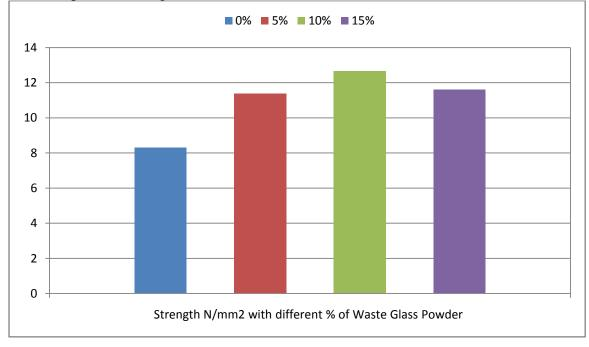
The compressive strength of Concrete cubes with 15% Glass Powder =  $11.6 \text{ N/mm}^2$
