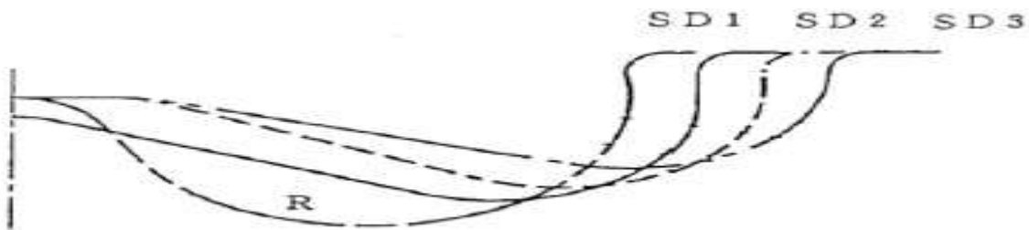
Fig.13. Comparison of combustion chamber shapes (Hiromi Kondoh et al.1994).
