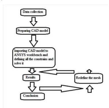
The important stages are creating CATIA model, defining constrains, results, redefining the mesh size and comparing results to the original results to validate the results and conclusion
