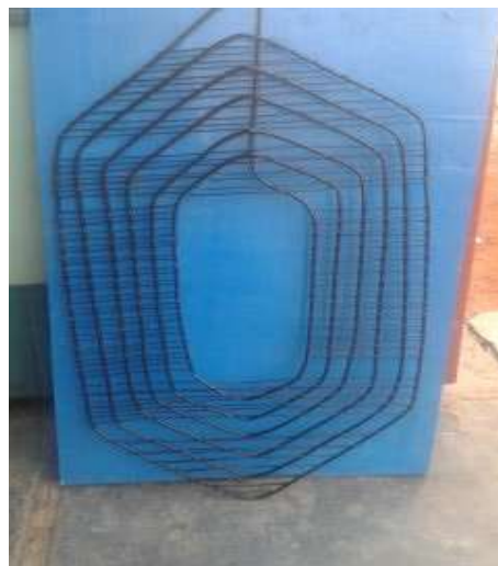
Fig.3.2 Hexagonal shaped condenser coil
