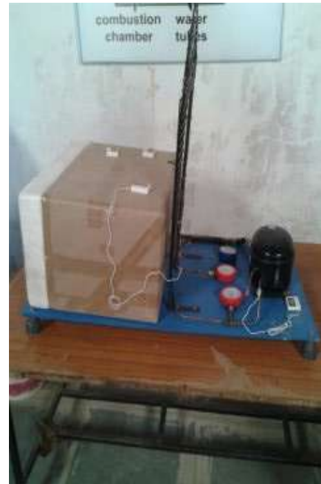
Fig.3.4 Hexagonal shaped condenser coil experimental setup side view
