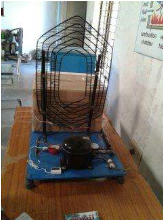
Fig.3.3 Hexagonal shaped condenser coil Experimental setup front view
