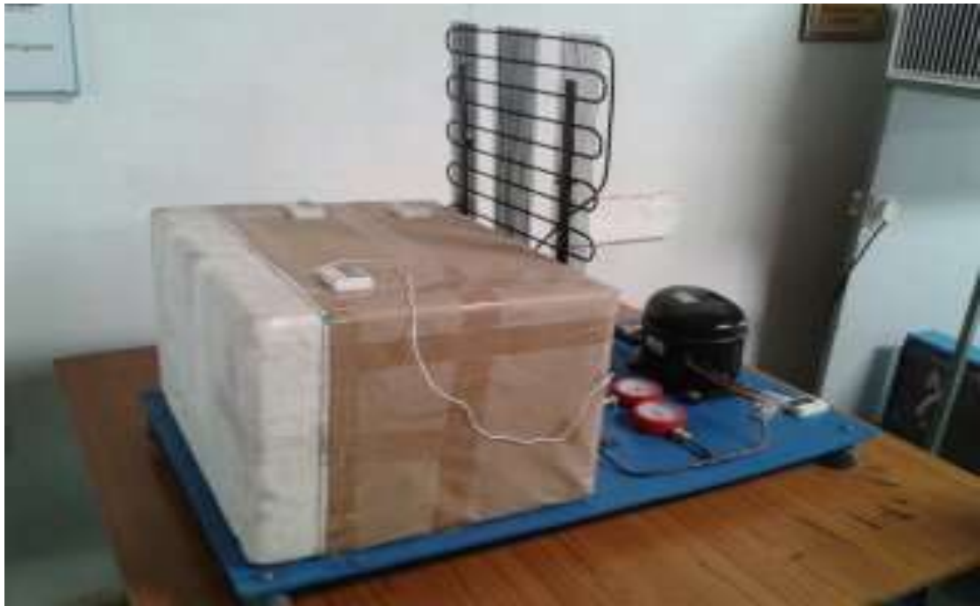
Fig.3.1 Conventional shaped condenser coil Experimental setup
