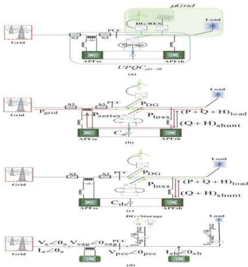
Fig. 2. (a) Integration technique of the UPQC $\mu$ G-IR. Working principle in (b) interconnected mode, (c) islanded mode, and (d) fundamental frequency representation.
