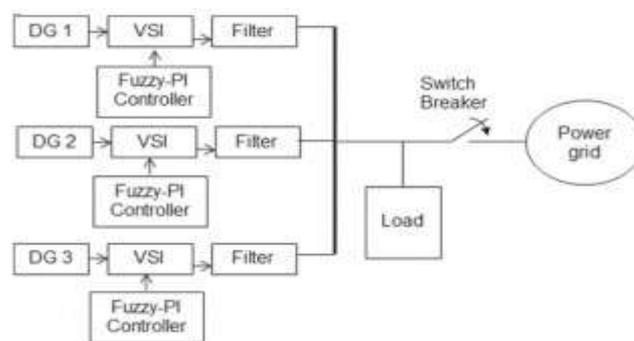
Fig.1. Block Diagram of the Micro Grid System
