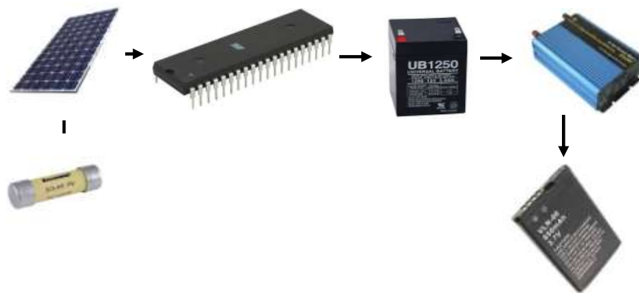
Fig. 2. 10 Volt Solar photovoltaic system for mobile phone charging.
