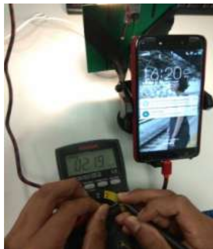
Fig.9. Operating Buck Converter measured current.
