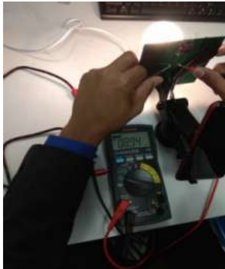
Fig. 6. Operating Solar Panel measured voltage.
