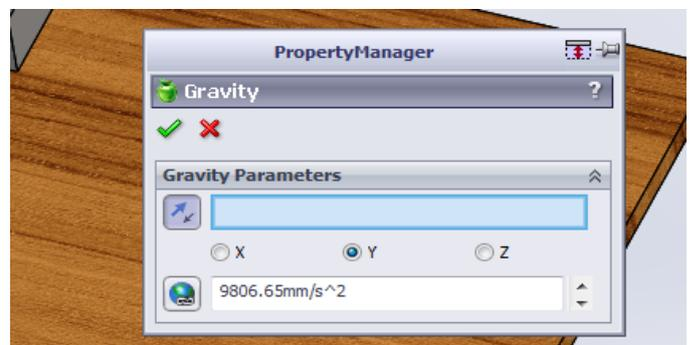
Fig.4: Apply gravity to the mechanism
