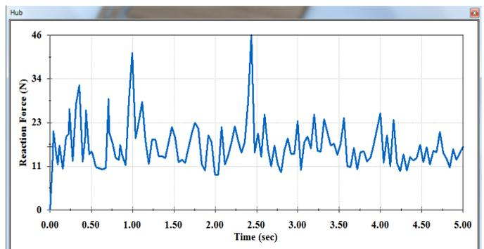
Fig.8: Reaction force on Hub Vs time at 120 rpm
