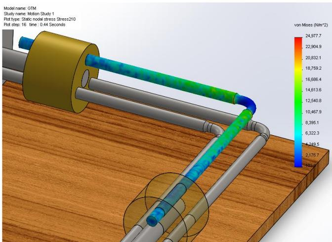
Fig.9: Distribution of Von Mises stress at 120 rpm
