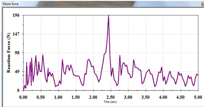
Fig.6: Reaction force on elbow rod Vs time at 120 rpm
