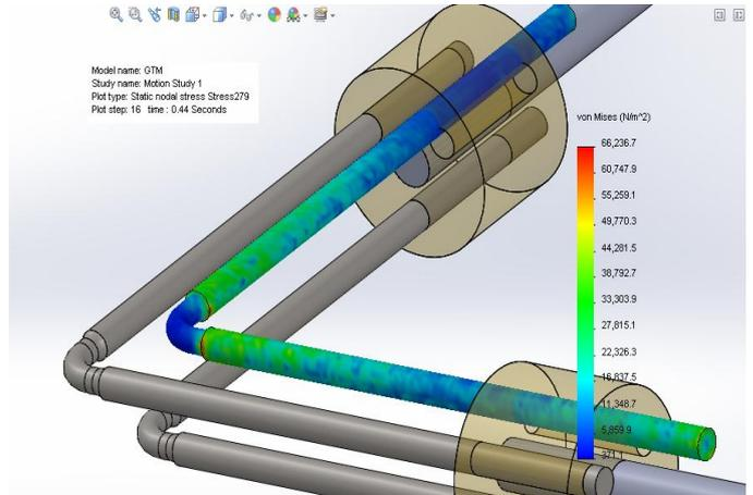
Fig.10: Distribution of Von Mises stress at 140 rpm
