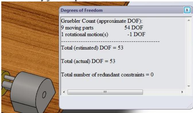
Fig.5: workbench snapshot of DOF & redundancies
