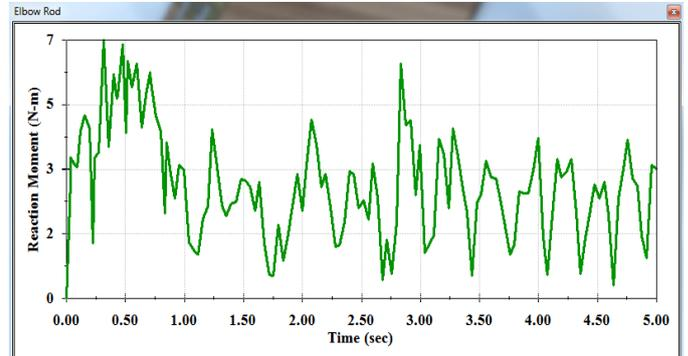
Fig.7: Reaction moment on elbow rod Vs time at 120 rpm
