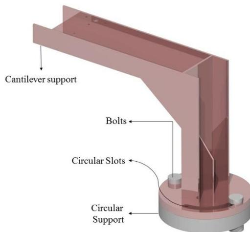
**Fig. 5: Rotatable Cantilever arm**
