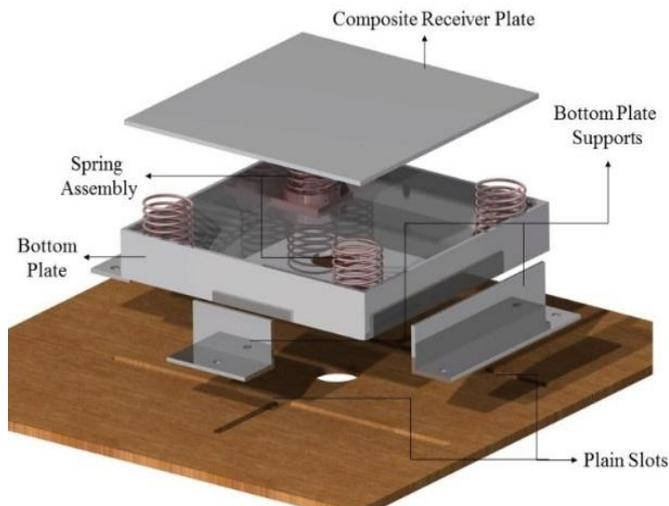
**Fig. 8: Variable sizes with spring assembly**
