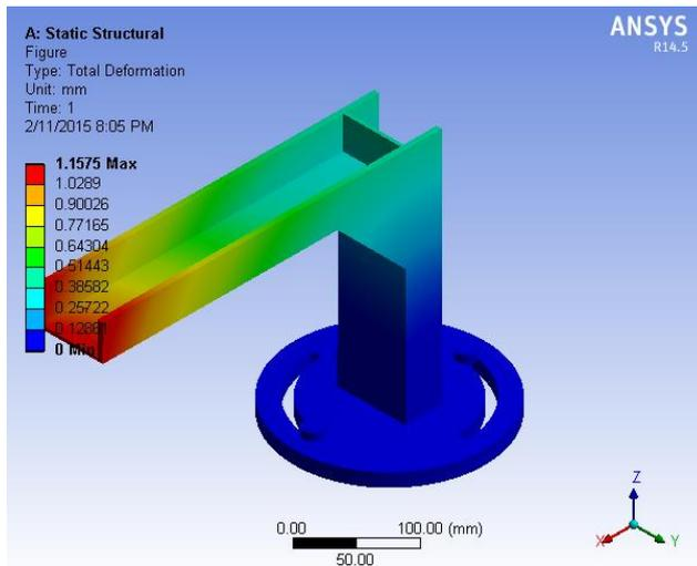
**Fig. 6: Total Deformation of Modified Design**
