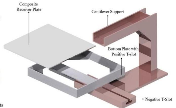
**Fig. 9: Sliding T-Slot assembly**
