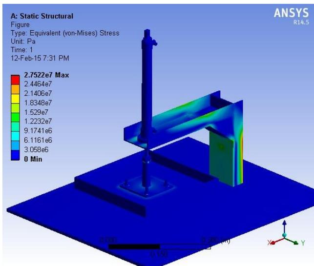
**Fig. 3: Stress Distribution of Initial Design**
