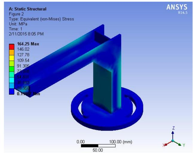
**Fig. 7: Stress Distribution of Modified design**
