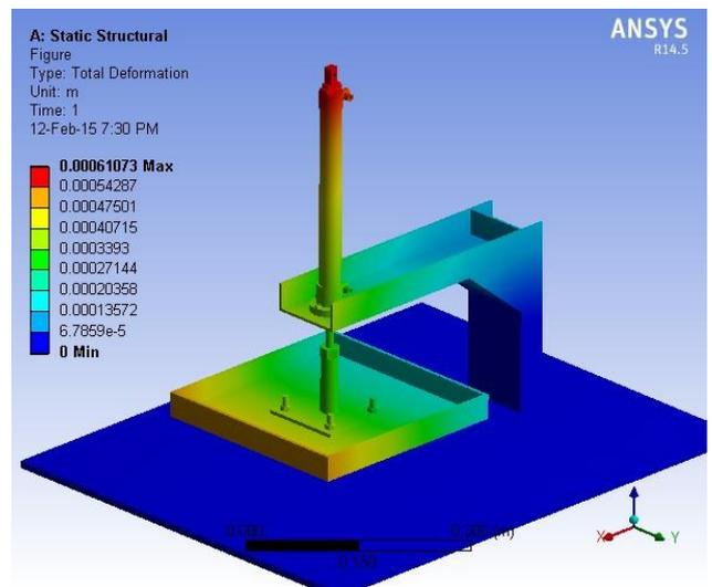
**Fig. 4: Total Deformation of Initial Design**
