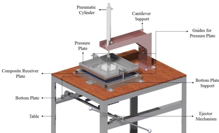
Fig. 1: Initial Design Assembly
