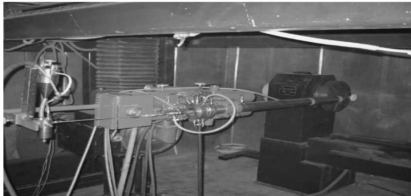
Fig.2. D-Gun method for thermal spray coating.
