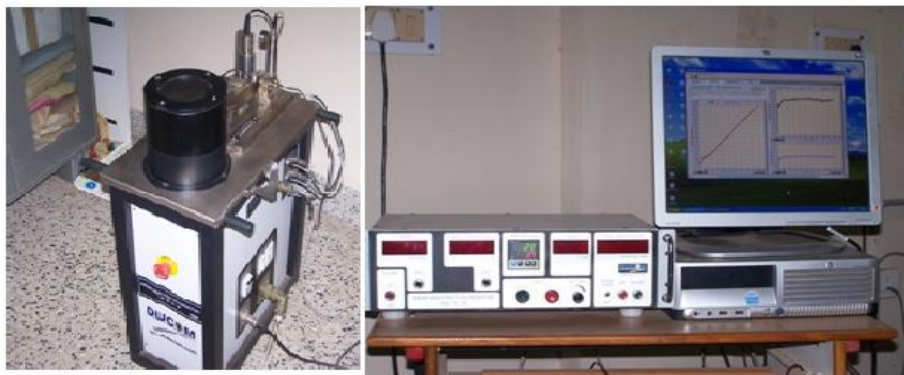
Fig. 3. Pin-on-disc method for wear testing
