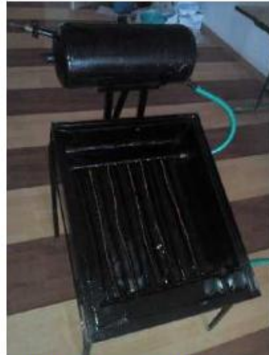
Figure 2: Solar Water Heater With Agitator
