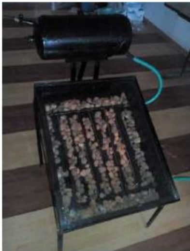
Figure 3: Solar Water Heater With Porous Medium
