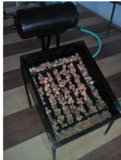
Figure 4: Solar Water Heater With Agitator, Porous Medium & Transparent Cover
