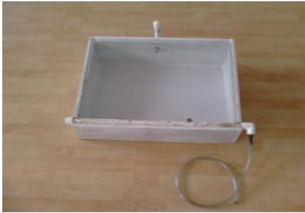
Figure 3. Solar Still with White Coating
