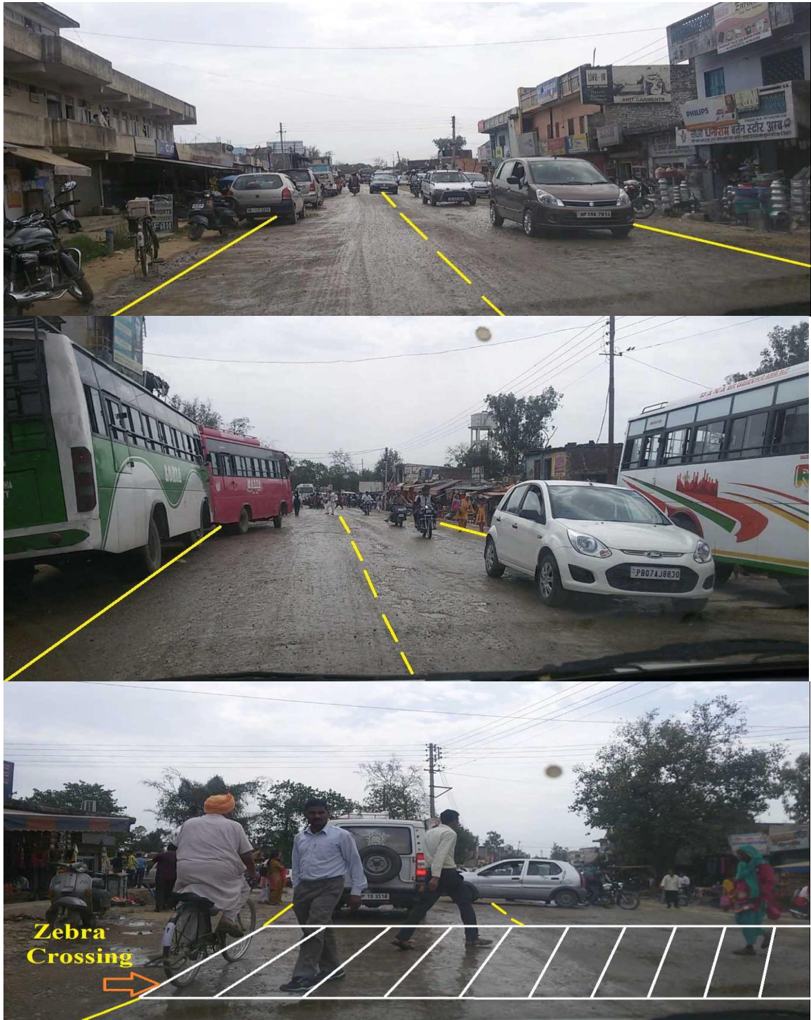
Fig 2.6: Suggestions for improvement for Amb city accident location. Source: Site visit photography.
