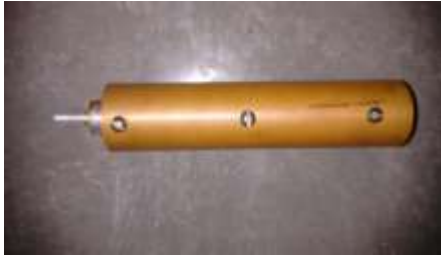
Fig 3.4(a) Composite pin fin (copper + Aluminium)
