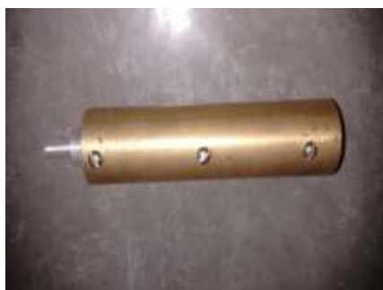
Fig3.3(a) Compositepinfin (brass+Aluminium)
