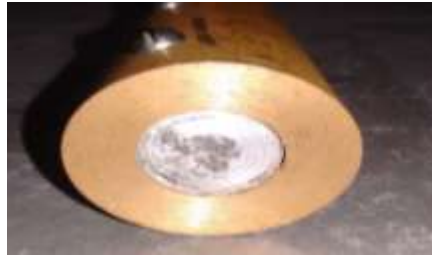
(b) Cross Sectional (Side View) View Of Composite Pin Fin (copper + Aluminium)
