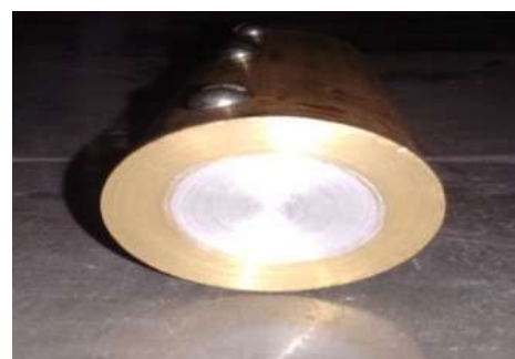
(b)CrossSectional(SideView) View Of Composite Pin Fin (Brass+Aluminium)
