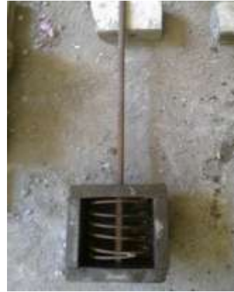
Fig. 4. Arrangement of Rebar & Helical Reinforcement
