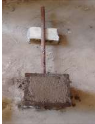
Fig.3. Pullout Test Specimen
