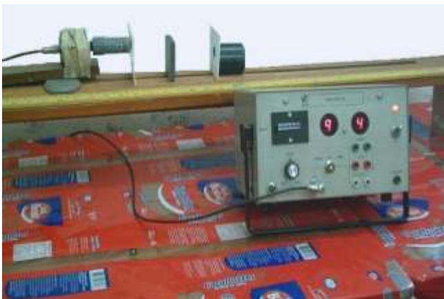
Figure:-03 Good or Narrow Beam Geometry
