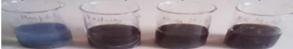
Fig. 4.4:- showing four different water samples containing K_2Cr_2O_7 when kept in water bath.
