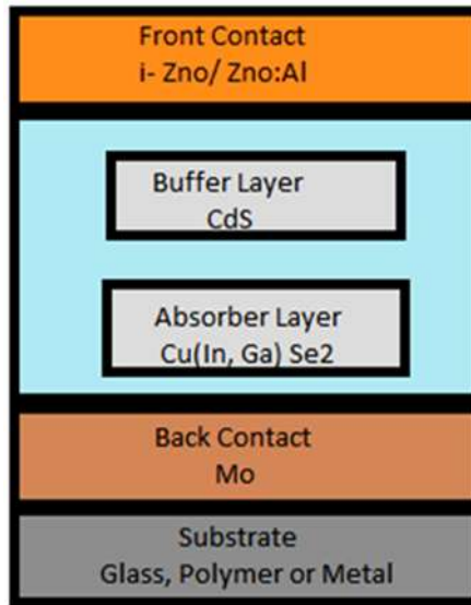
Figure 6: Standard structure of CIGS solar cell
