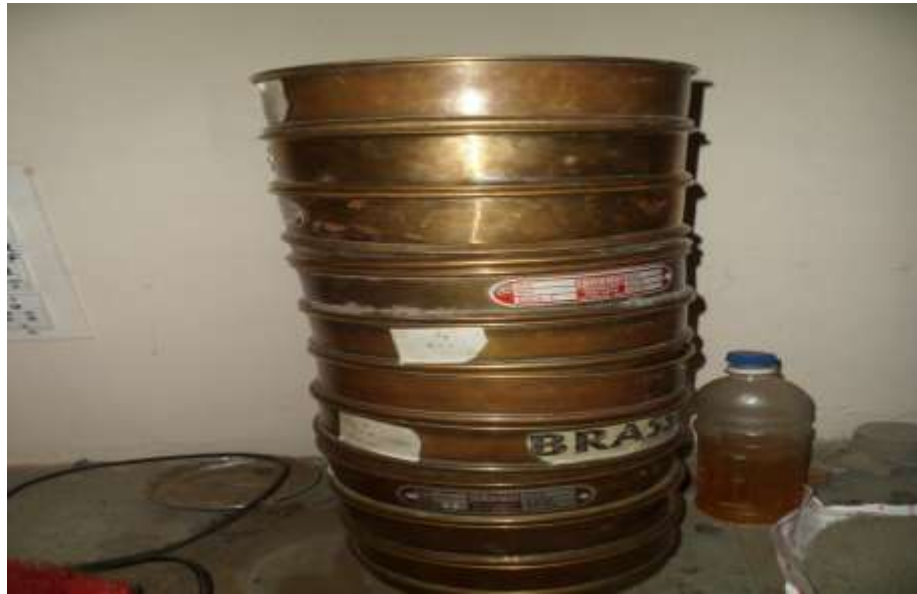
Figure1. Sieve Apparatus for Particle size analysis
