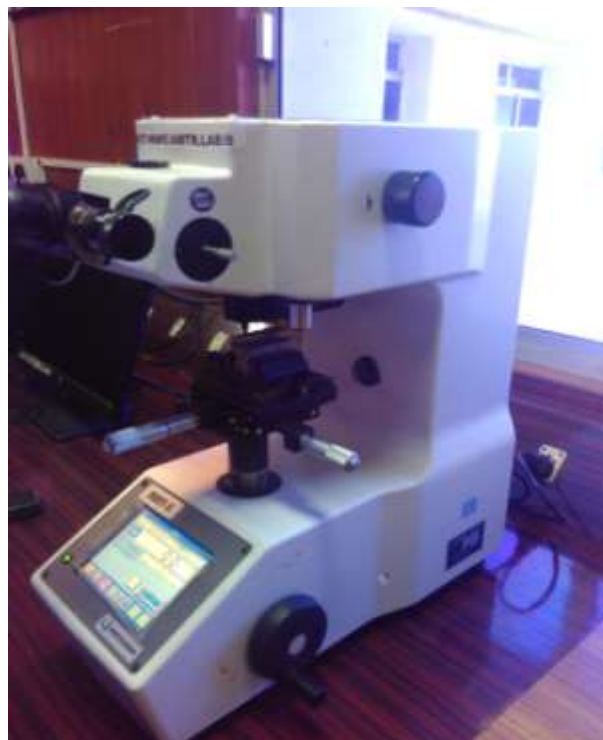
Figure 8: Matsuzawa microwickers hardness testing
