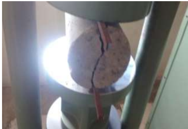
Fig.No.3. Split Tensile Test on Cylinder
