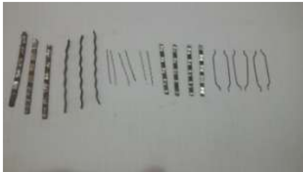
Figure1. Different types of steel fibres used in HSFRC
