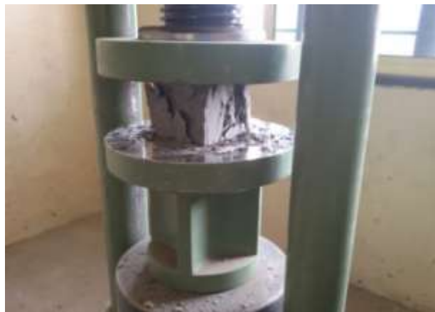
Fig. No.2. Compressive Test on Concrete Cube
