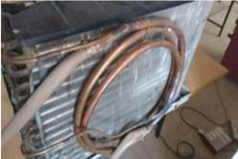
Fig No: 4.1 co-axial copper pipe
