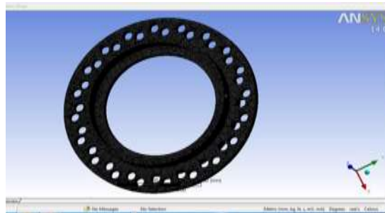
3-D Meshed Model by ANSYS
