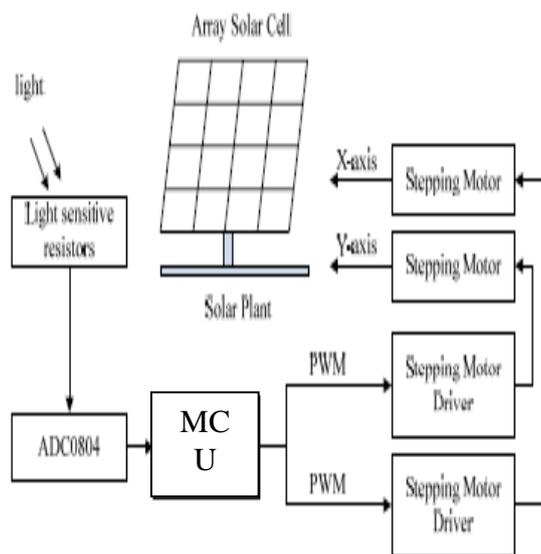
Fig. 2. System architecture of the solar tracking system.
