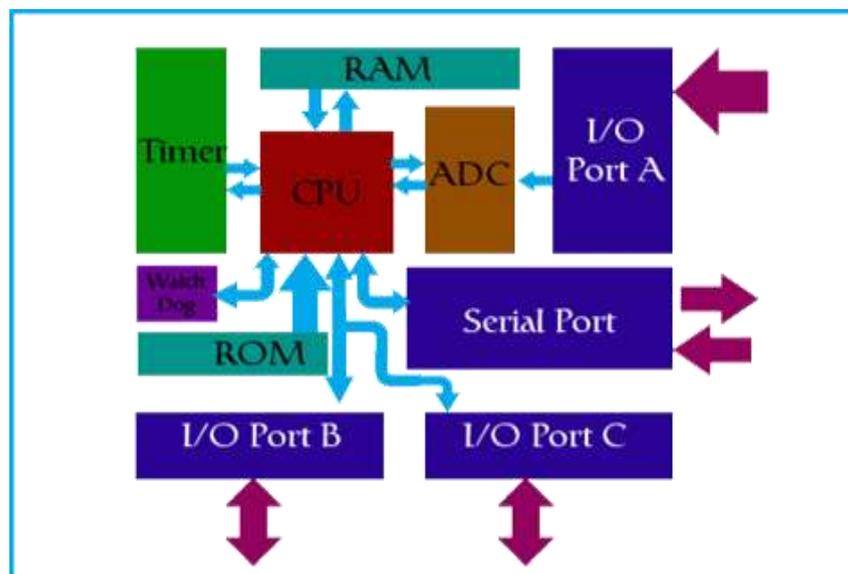
Figure-Block Diagram of Microcontroller (AT89S52)
