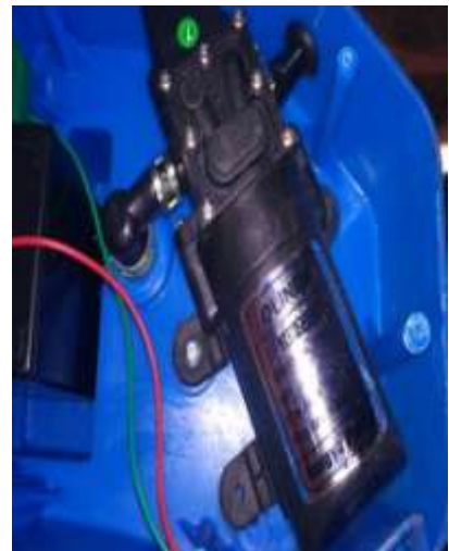
3. DC water pump
