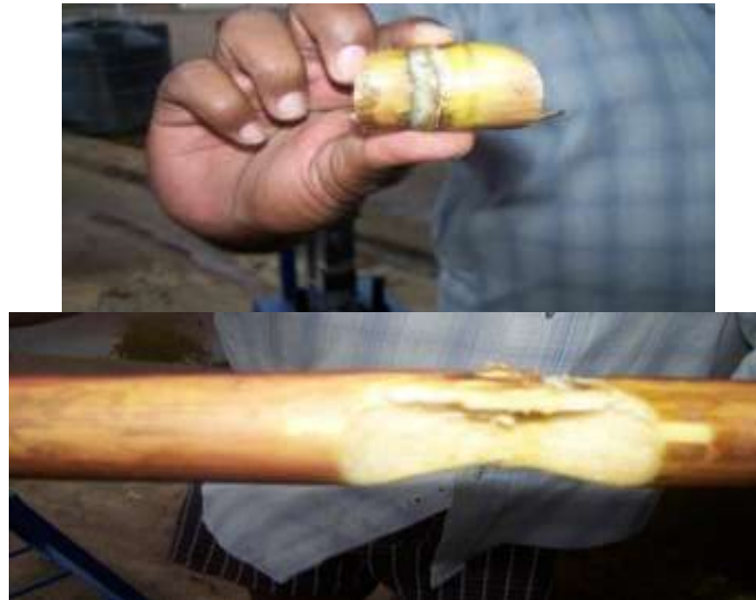
Figure 3. Cutted Sugarcane Buds By Machine
