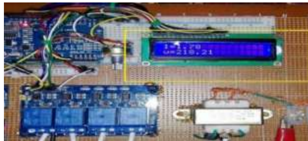
Figure (14) practical reading of current and voltage
