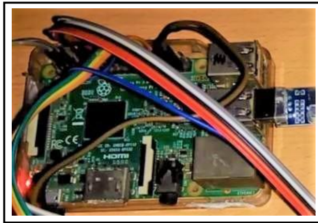
Fig II: Raspberry Pi 3B+ as the main Controller
