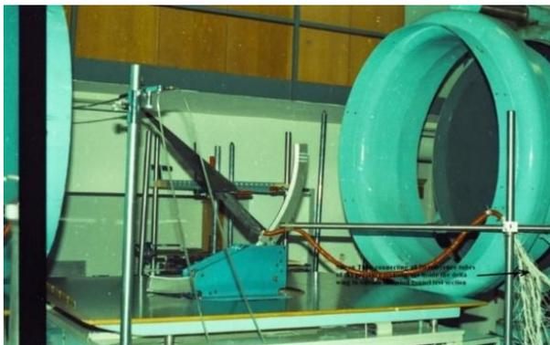
Figure 8: The delta wing in the wind tunnel
