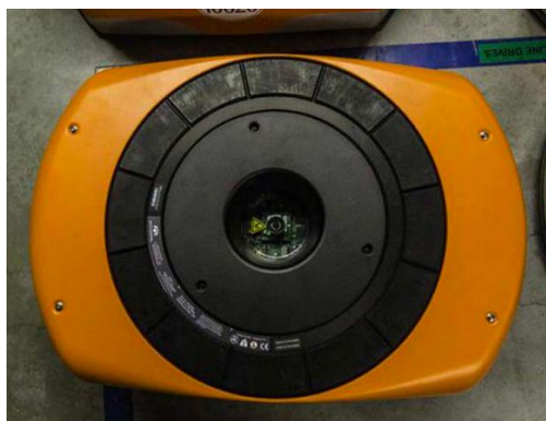
Fig. 1. Camera-equipped Kiva robot in Amazon warehouse[1]
