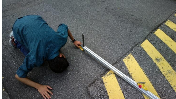
Figure 10: Measuring bump height
