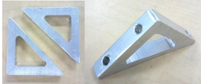
Figure 22: Fabricated vacuum pump holders
