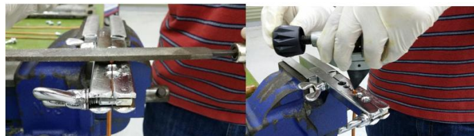
Figure 23: Filing & chamfering brake lines
