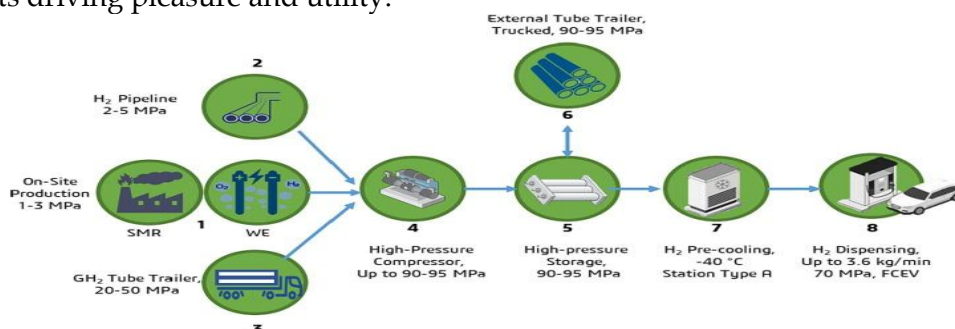
Figure 7: Hydrogen refueling station: Overview of the technological status and research enhancement
