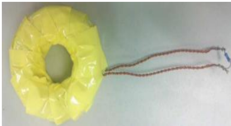
Fig. 4. A Prototype of HFCT sensor developed
