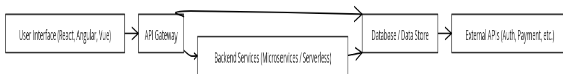
Figure 2. Typical Modern Web App Architecture featuring a front-end framework communicating with microservices via an API gateway, with external APIs for specialized services (e.g., authentication, payment).
