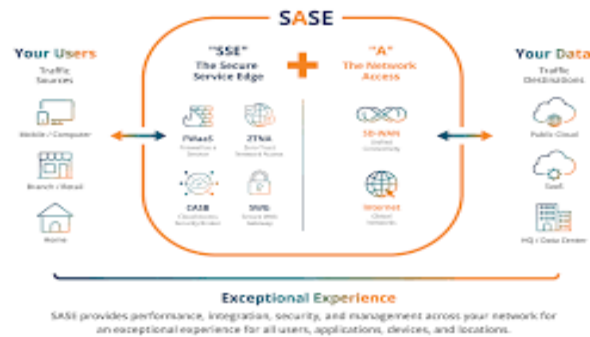
Figure 4: Secure Access Service Edge (SASE) architecture
