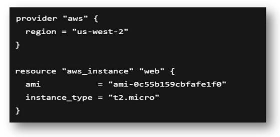
Figure 2: Launching an AWS EC2 using Terraform
