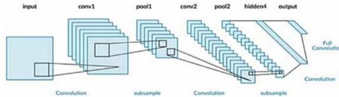
Fig. 2. Semantic segmentation convolution neural network
