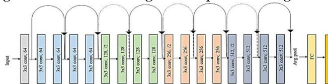
Fig. 4. Original ResNet-18 Architecture
